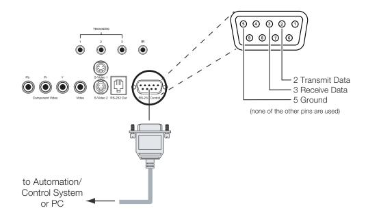
Figure 3-9. RS-232 Control System Connection
